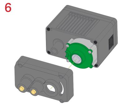
Ensure gear cartridge is seated properly.
