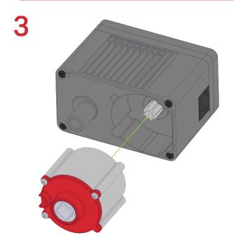
Remove gear cartridge from motor housing.
