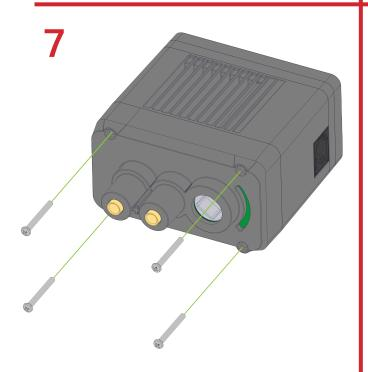
Insert (4) screws into motor housing.
