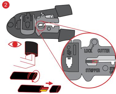
To cut to length, insert the V5 Cable Stock underneath the cutting blade. Squeeze the crimping tool firmly to cut the cable.
