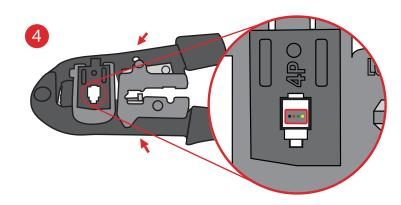
Insert the connector into the crimping tool and squeeze firmly.
