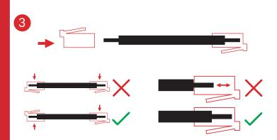
Insert connectors on each side of the cut cable. Ensure that cables are fully seated inside connector, and that they are correctly oriented.
